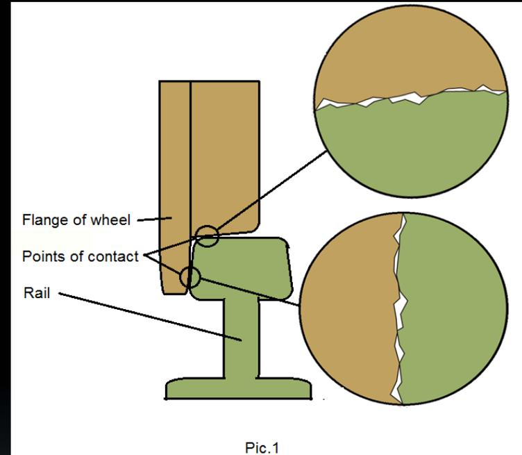
Reducing the coefficient of friction is only one feat to accomplish, without increasing the hardness of the metal we are only halfway there
