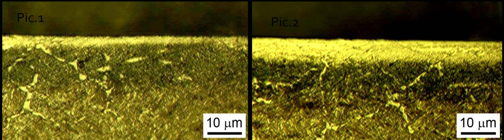
The new smooth tribo-layer can be seen in picture 2 through an electronic microscope. This new nanoceramic surface is formed by a chemical interaction between the nano-compound and host metal preventing metal to metal contact.
